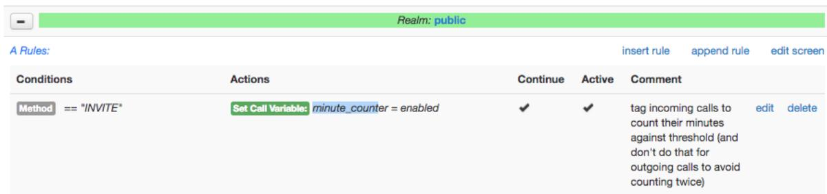
Fig. 38: Setting Minute Counter Call Variable
